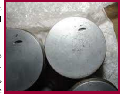
This piston crown shows pitting likely due to detonation or early combustion.
